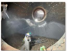
thickness allows for ample abrasion and corrosion protection with minimal dimension changes to the sag mill. This application provides a seamless liner that will outlast the rubber that it replaced. ShieldPoly has an excellent combination of high tensile strength, high elongation, and high hardness
